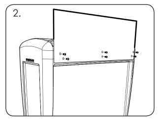
Position the sign carrier (item 1) and align the six fixing holes on the rear of the unit.
