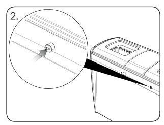
To lock, twist 45 degrees anti-clockwise and push the barrel inward.
