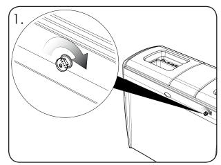
To unlock, twist key to 45 degrees clockwise until the barrel retracts.
