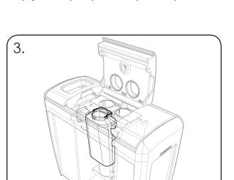
Empty the liquid reservoir by lifting it from the unit by the carry handle. Pour away the contents.
