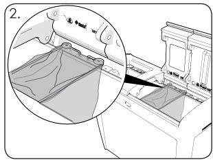
Step 3 - Stretch the sack over the rear upstands and hold in place with the bungee.
