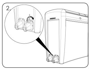
Insert screws (Item 2) through holes and tighten using Allen Key (Item 3).
