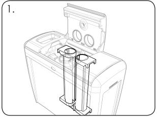
To Remove the cup stacker from the unit to empty the cups, open the aperture panel.
