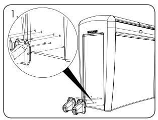
Line up wheels (Item 1) with fixing holes on side of the body.
