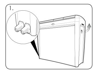
Use the handle to lift and tilt the bin until the wheels touch the ground allowing bin to be manoeuvrable.
