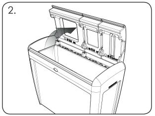
Open the lid to 90 degrees by pushing past the bump feature until the lid rests in an upright position. To close the lid pull the front down firmly to override the bump feature.
